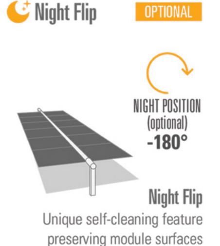
preserving module surfaces from dust and soiling
