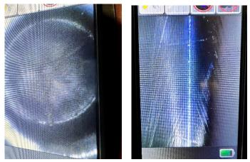
Hatch marks are still clearly visible, and no signs of glazing have developed despite conditions of engine use. Piston crown is showing a nice clean burn pattern and minimal carbon deposits.
