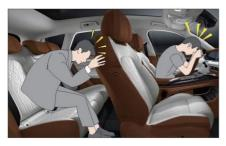
In the event of a vehicle collision, the driver and occupant who are not wearing seat belts may be thrown out of the vehicle and injured due to inertia. Even if the vehicle speed is very low, the force acting on human body during a collision is very large, and a secondary collision is very likely to occur.
