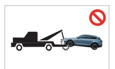
The vehicle should be towed with four wheels lifted off the ground and hauling is prohibited.
