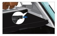
Removal: after folding the curtain, hold the fixed clips at both ends of the curtains, compress the fixed clips inward to remove the curtain.
