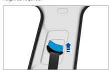
Move down: Press the release button of the height adjuster and move it downward (in the direction indicated by the arrow in the figure below), adjust the shoulder belt to an appropriate height as needed, and then release the release button. When vou hear a "click" sound, it means the adjuster is locked.
