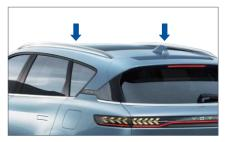
In order to avoid damaging the roof, please use the lateral support rods approved by VOYAH.
