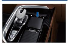
The touchpad is located on the right side of the shift lever, and it is mainly used to recognize various gesture information to perform corresponding operation functions:
