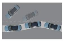
Vehicles not equipped with ESC may skid off the normal driving route when running.
