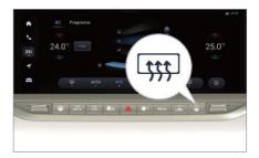
Press the heating button of the exterior rearview mirror, the button indicator goes on, and the heating function of the exterior rearview mirror is turned on. which can remove the fog or frost on the exterior rearview mirror and the rear windshield. Press the button again to turn off the heating function. The button indicator goes off.
