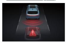
RCW detects the distance between the vehicle behind and the subject vehicle through radar. When the vehicle behind is fast and may have a rear-end collision with the subject vehicle, the subject vehicle emits a warning sound and the instrument cluster issues a warning message to remind the driver that a rear-end collision may occur. At the same time, the hazard warning lamps flash rapidly to warn the vehicles behind to keep a safe distance.
