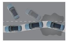
When the vehicle accelerates rapidly or starts on a low-adhesion road, the driving wheels may idling in place, affecting the stable driving of the vehicle. The traction control system (TCS) can effectively prevent such phenomena by controlling the driving force of the wheels.
