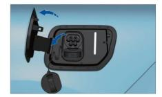
2. Connect the charging plug that comes with the charging pile to the AC charging port of the vehicle;
