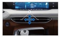
Move the grille up, down, left and right to adjust the air outlet direction, and move it to the left/right end to close the air outlet.
