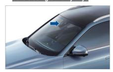
The position of the rain and light sensor is shown by the arrow in the above figure. When the rain and light sensor detects rain, the windows and sunroof will be automatically closed.
