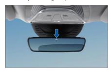
The vehicle is equipped with automatic anti-glare interior rearview mirrors. When driving at night, if there is strong light behind, the interior rearview mirror will automatically adjust the mirror reflectivity to reduce the reflection of the strong light.
