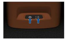
There are USB Type-A and Type-C interfaces in the rear row. The former supports QC3.0 18W for charging and the latter supports PD 60W for charging; both interfaces do not support data transmission.
