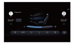
In the dual zone control mode, the temperature of the driver zone and the front passenger zone can be adjusted separately:
