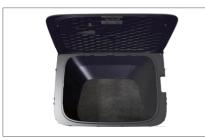
The front trunk (for EV) is located in the engine compartment. Open the engine hood and pull the front trunk release handle to open the front trunk, which can be used for loading items.
