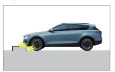
When going down a steep slope, the vehicle head hits the ground.
