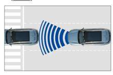
Front vehicle start reminder (FVSR) is a driving safety assistance function, and the following conditions must be met to trigger the FVSR function:
