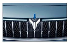
The front view camera is located above the front bumper logo and is used to record the area in front of the vehicle.
