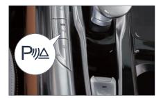
The front PDC is turned on by default after the vehicle is started. You can turn on/off the PDC through the PDC switch beside the shift lever.
