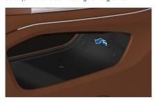
3. Remove the new fragrance protective film, put in the new fragrance, and refit the fragrance plug and storage box pad.
