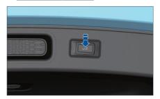
Press the POT inner closing switch to close the POT. At any height, press and hold the POT closing switch to set the current height as the POT opening height. In this case, the buzzer sounds for a long time, indicating that the height setting is successful.
