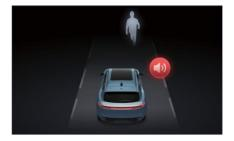
When the vehicle is running at a low speed, the lowspeed pedestrian warning system will issue a warning sound for pedestrians approaching the vehicle to warn pedestrians to pay attention to safety.
