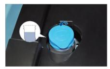
The windshield washer fluid unit is located in the engine compartment. When the washer fluid is insufficient, the low washer fluid level indicator in the IC will light up and display "Low washer fluid level" to remind you to add it in time.
