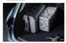
The rear trunk can load larger items. To ensure stable and safe driving of the vehicle, when loading luggage, items should be placed as evenly as possible, and heavy objects should be placed at the front of the trunk.
