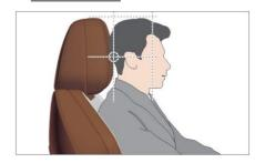
Correctly adjusting the height of the head restraint is essential to protect the safety of the driver and passengers. When adjusting the head restraint, the upper edge of the head restraint is flush with the edge of head.
