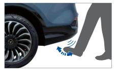
Approach the vehicle identification area with the smart key, then kick your toes into the middle of the rear bumper at least 10 cm, and the POT can be opened/closed.
