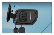
2. Connect the charging plug that comes with the charging pile to the DC charging port of the vehicle;
