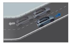
Hill start assist (HSA) can prevent the running vehicle from slipping backward when starting uphill, or sliding forward when reversing downhill. During this process, the driver does not need to operate the EPB button, thus effectively reducing the difficulty of starting or reversing on the slope.
