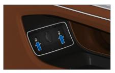
There are two USB Type-A interfaces under the front central armrest with the charging power of 10.5 W, which supports data transmission.
