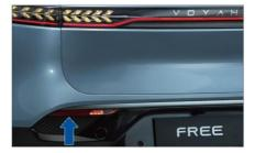
The rear retro-reflecting device is used to reflect the light from the vehicle behind, reminding the driver of the vehicle behind to keep a safe driving distance.
