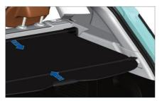
Unfolding: pull the curtain handle backward to fix the curtain in the grooves on both sides of the body.
