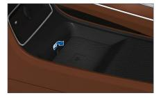
2. Remove the fragrance plug at the rear of the console (as shown by the arrow in the figure below), and take out the original fragrance
