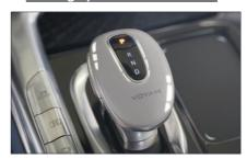
The vehicle has four gears: P, R, N, and D. After the vehicle enters the READY state, depress the brake pedal and switch gears, the corresponding gear light on the shift handle will light up, and the corresponding gear will be displayed on the instrument cluster.
