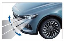
The AFS automatically adjusts the illumination angle of the headlamp according to the load status of the vehicle (no-load, light-load, medium-load, full-load) to ensure a suitable illumination range.
