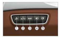
The light combination switch is located on the left side of the instrument panel.
