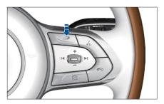
The display information of the instrument cluster can be switched by the menu button— on the steering wheel, to view the current vehicle tire pressure and temperature.
