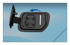
Swipe right on CSD interface to show the -1 screen, touch the Open C. Port, and the charging cover will automatically pop open. After the charging cover is opened, you can manually press it inward to close it.
