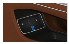
The front 12V power interface is located under the central armrest and can be used when the trim cover is opened. The maximum allowable power is 120W.
