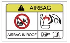
A warning label is attached to the right sun visor to remind the front row occupants of the danger of deploying the frontal airbag. Please read and follow the instructions on the label.
