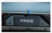
The rear license plate lamp is installed next to the rear view camera to illuminate the vehicle license plate.
