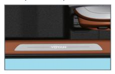
Side step welcome lamp is located on the door sill to provide illumination for occupants when getting on and off the vehicle.
