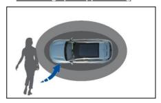
When you approach the vehicle with the smart key, the door will automatically unlock, the left and right turn signal lamps will flash twice, and the exterior rearview mirrors and concealed door handles will automatically deploy.
