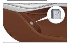
When the vehicle is stationary, lift up the driver side POT switch, and the POT can be opened; press the driver side POT switch , and the POT can be closed.
