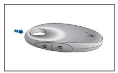
2. Open the smart key back cover, and take out the exhausted battery;
