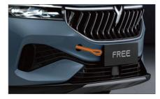
4. Connect the trailer connection device. It is recommended to use the hard connection method first. The tow rope can only be used if there is no drawbar.
