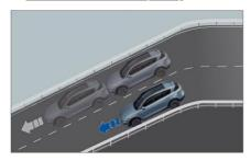
Hill descent control (HDC) can be used to actively brake and decelerate when the vehicle is passing through a steep downhill section, so that the vehicle can move safely and smoothly.
