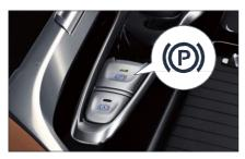
Activation: After the vehicle is stopped, lift up the EPB button / press the P gear button, the EPB indicator and button indicator on the instrument cluster will light up, and EPB will be activated.
