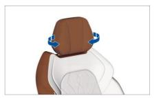
Adjust the wings on both sides inward and outward.
