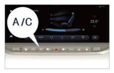
Press the A/C cooling button, the button indicator will go on, and the A/C system will activate the cooling function.
