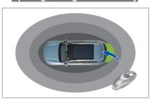
Approach the vehicle identification area with the smart key, and press the smart key POT button twice in a row to open/close the POT.
