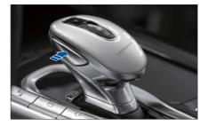
When switching out of P gear or switching into R gear, you need to press the unlock button on the side of the shift handle (as shown by the arrow in the above figure).
