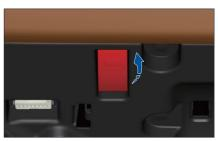
Pull the engine hood opening handle twice in a row and lift the engine hood to open it. After the engine hood is opened, the above message will appear in the instrument cluster.
