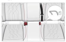
Place the child safety seat on the seat, find the lower fixing point ①, and insert the lower mounting slot (as indicated by the arrow in the above figure) of the child safety seat into the lower fixing point ① in the gap of the seat cushion until an engagement sound is heard;
