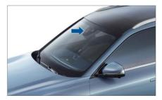
The automatic light sensor is located in the upper middle of the front windshield, do not cover this part and keep it clean so as not to affect the automatic light control function.
