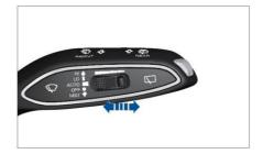
When the wiper stalk is in the AUTO position, turn the knob to the left to increase the auto wiper sensitivity; turn the knob to the right to reduce the auto wiper sensitivity.
