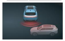
When the vehicle shifts into the R gear (reversing), the RCTA detects through the radar that there are pedestrians, moving vehicles or moving objects approaching on the left and right sides of the rear of the vehicle, and there is a risk of collision, the CSD will prompt an alarm message, accompanied by a warning sound, to remind the driver to avoid safety accidents.
