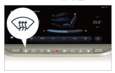
Press the front windshield defogging button, the button indicator will go on, the front windshield defogging function will be activated, and the system will automatically perform the following settings:
