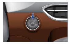
The vehicle is equipped with a START/STOP button. The START/STOP button can only be operated when the vehicle detects the smart key.
