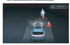
The NVS provides clear images at night and displays detailed information of the road, such as pedestrians, vehicles, lane markings, traffic signals, etc., thereby providing drivers with more comprehensive and accurate road information and issuing hazard warnings in advance.
