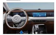
Footwell lamps are installed in front of the driver and the front passenger to provide illumination for the front row personnel when getting on and off the vehicle.
