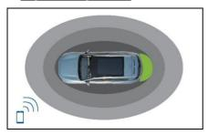
When approaching the vehicle with the smart key, press the POT switch, and the POT can be opened.
