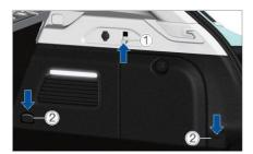
Hooks (1) on the left and right sides of the trunk can be used for lighter items. Fixing rings 2 on the left and right sides of the trunk can be used to bundle and fix larger items placed in the trunk.
