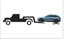
A towing trolley is placed under the rear wheels of the towed vehicle.
