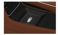
When the power of the smart key is low, you can put the smart key in the emergency start area (shown by the dotted line in the figure above), depress the brake pedal, and press the START/STOP button for emergency start of the vehicle under the premise of ensuring all the doors and the POT are closed
