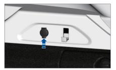
The rear 12V power interface is located on the right side of the rear trunk and can be used when the trim cover is opened. The maximum allowable power is 120W.
