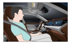
Sit as fully as possible in the seat, keeping your back and shoulders in line with the seat backrest, and adjust the height of the head restraint so that the upper edge is level with your head.
