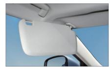
Detach the sun visor from the bracket and turn it to the side to block sunlight from the side.
