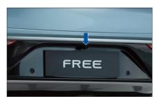
The rear view camera is located next to the license plate lamp in the rear bumper and is used to record the area behind the vehicle. When R gear is engaged, and the reversing dynamic assist line will be shown on the display.
