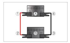
When connecting the batteries of the two vehicles, the positive terminal must be connected first, and then the negative terminal:
