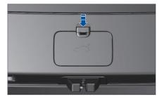
4. Press down the emergency switch and push the power tailgate outwards.
