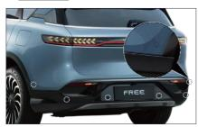
The rear PDC is mounted on the rear bumper of the vehicle.
