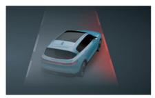
Lane keeping assist includes three safe driving assist functions: Lane departure warning (LDW), Lane keeping assist & departure warning (LKA) and Lane centering control (LCC).
