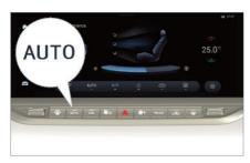
Press the auto mode button, the button indicator will go up, the A/C system will enter the automatic mode, and the following items will be automatically controlled according to the set temperature value:
