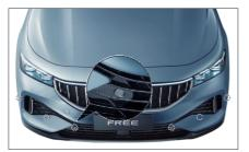
The front PDC is mounted on the front bumper of the vehicle.
