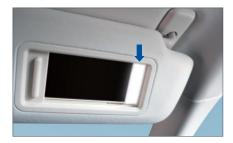
Open the sun visor and pull the trim cover, the makeup mirror lamp will be automatically turned on; close the trim cover, the makeup mirror lamp will be automatically turned off.
