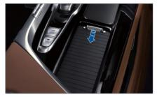
The front cup holder is located at the right of the shift lever, and the water cup can be placed after pulling the cover back.
