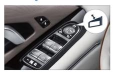
Press the button shown in the figure to unfold/fold the exterior mirrors electrically.
