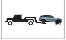
A towing trolley is placed under the front wheels of the towed vehicle.
