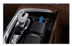
The mobile phone wireless charging induction area is located at the front part of the instrument panel (as shown by the arrow in the figure above). On >> Settings Device interface of the CSD, set the on/off function of Wireless Charging For Mobile Devices.
