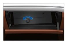
The glove box air outlet switch is located in the alove box.
