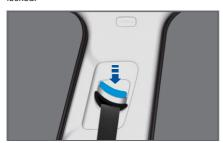
Without pressing the button, try to move the height adjuster downward to check whether the adjuster is locked in place.
