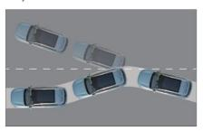
Vehicles not equipped with ABS may lose steering ability when the front wheels lock up. When the rear wheels lock up, the vehicle may drift.
