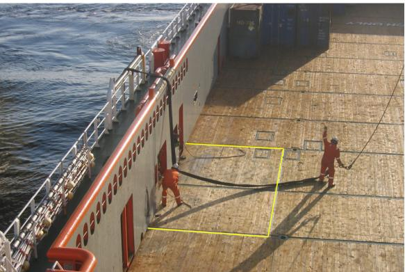
Securing after the hose has been landed avoiding the need to walk under a suspended load.
