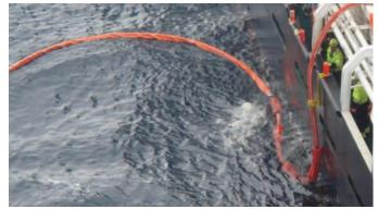
Sections of hose strings with integral buoyancy are also available and eliminate the need for floatation aids to be used.
