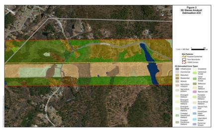
High resolution wetland mapping along a 450 mile pipeline corridor with limited access, using a 3D image analysis.
