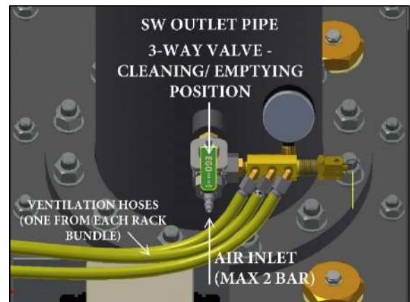
Cleaning/ Empty the Rack case for SW
