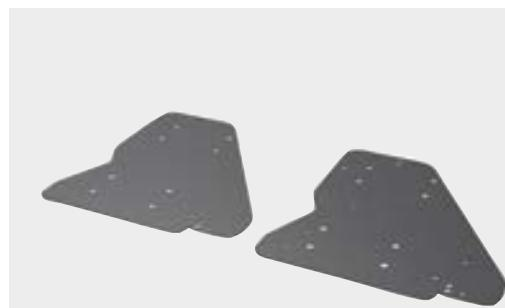
This article is used to enable the CONERO clothes lifts to be installed in an existing row of holes. This includes wardrobes with honeycomb panels (e.g. IKEA® PAX). The row of holes itself must be embedded in a load-bearing, torsion-resistant solid material (e.g. solid wood, chipboard). ATTENTION: Without this adapter plate, CONERO clothes lifts may only be installed in solid material (chipboard, wood or similar).
