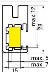
Permissible LED strip dimensions for use with LED adaptation plate
