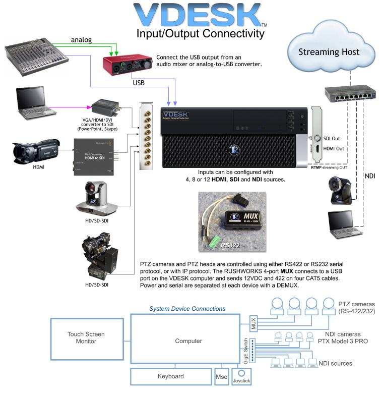
VDESK PRO systems are available with 4 inputs, 8 inputs, or 12 inputs (SDI or HDMI), NDI inputs and output, and HDMI / SDI outputs.
