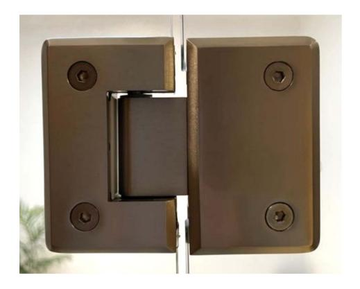
2 Each hinge has six hex-screws that need to be checked and re-tightened. The first four are located on the inside of your sauna. Using a torque-wrench set to 7.5 Nm, tighten these four screws until the torque wrench clicks.
