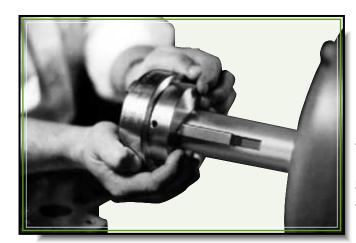
Shaft spacing should be within range given by dimensions 'W' and 'X' as shown in charts on page 4. Position each hub on proper size shaft - Magnaloy couplings are bored to standard "push fit" tolerances, if a tight fit exists check shaft for burrs. Maximum benefits are obtained with hubs posi-tioned to allow complete shaft engagement within bore. However, some equipment designs do not permit this condition - maximum shaft engagement should be utilized in any case.
