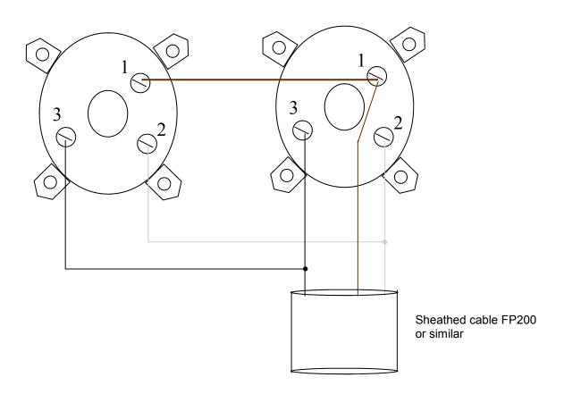
With the above wiring layout you would connect the grey and black into air pressure switch terminals 3 & 3 on the PCB as normal. These connections would in effect be the actual interlock.
