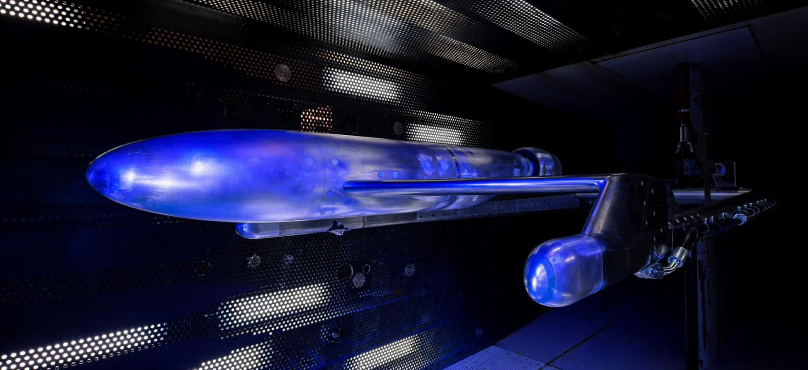
Having previously investigated the potential of a steel wing with the founders of WAAM3D and their team at Cranfield, the aerodynamics engineers at ARA knew that WAAM had the potential to reduce wind tunnel model lead times and costs.
