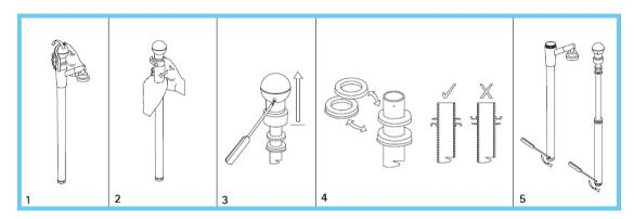
Should the Drumpump fail to pump, replace the valve flaps. Ask for Ezi-action® Service Kit (Refer Steps 5-9)
