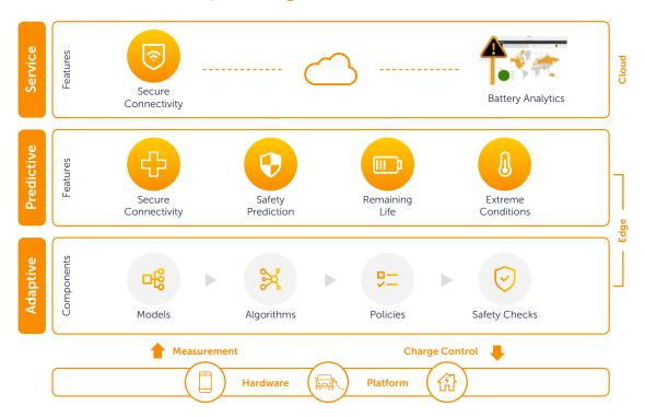
Adaptive charging algorithms combine requisite diagnostics with learning chemical mod-els to maximize battery life and longevity. Qnovo's technology analyzes the battery's in-ternal chemical processes. By studying the state of battery health and anticipating future aging, it dynamically adjusts the rate and degree of charging to meet some of the most challenging requirements such as those demanded by 5G smartphones.
