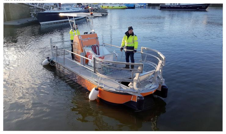
The Waste Cleaner 66E is a 100% electric clean-up and depollution vessel with unique and innovative technology for the collection of solid and liquid floating waste including hydrocarbons.
