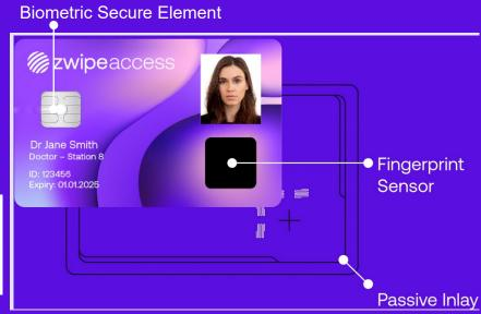
**Zwipe Access** is a card-based fingerprint access control solution. Fingerprint capture, extraction, and comparison are performed within the Zwipe Access card. This means that the cardholder's biometric data never leaves the card providing increased data privacy to the cardholder.
