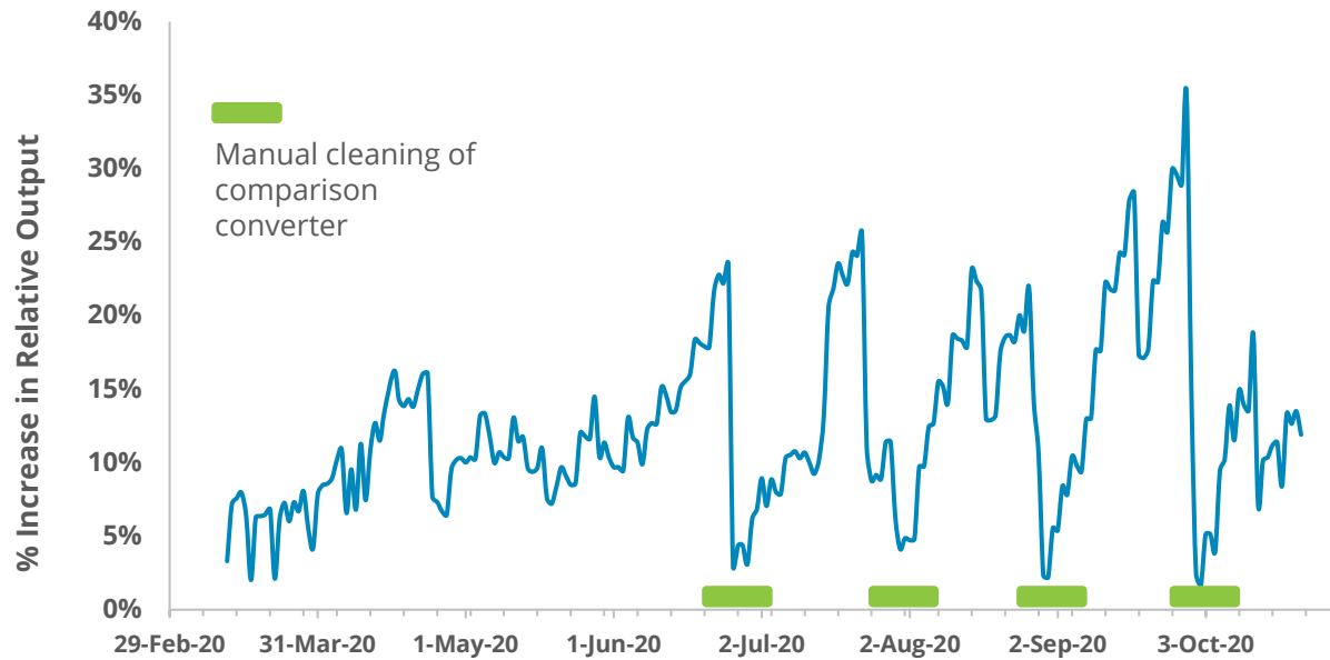
Improved production with RST compared to a system with manual cleaning
