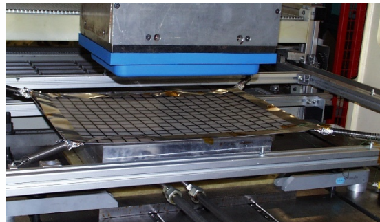
Curv® sheet held in sprung frame during heating and molding cycles
