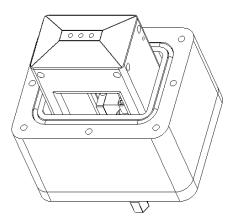
Figure 2. Three-dimensional mechanical design diagram of the plasma flood source
