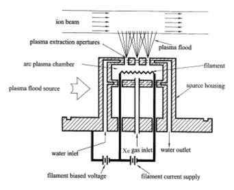
Figure 1. Functional block diagram of a plasma flood source.
