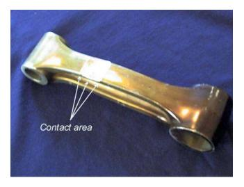
The owner is often unaware that a problem exists but such an engine is headed for a catastrophic failure when the bent link rod finally flexes in two.
