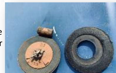
Figure 2-The failed back flow valve assembly on the right compared with the new assembly on the left.
