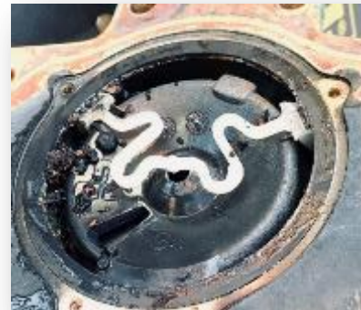
Figure 1-Example of debris found in 4 meters
