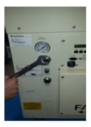
Figure 11 Remove Supply Coupling Locknut
