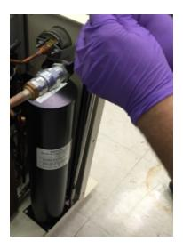
Figure 10 Disconnect Adsorber from Base
