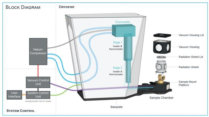
Figure 2: Cryostation connections overview
