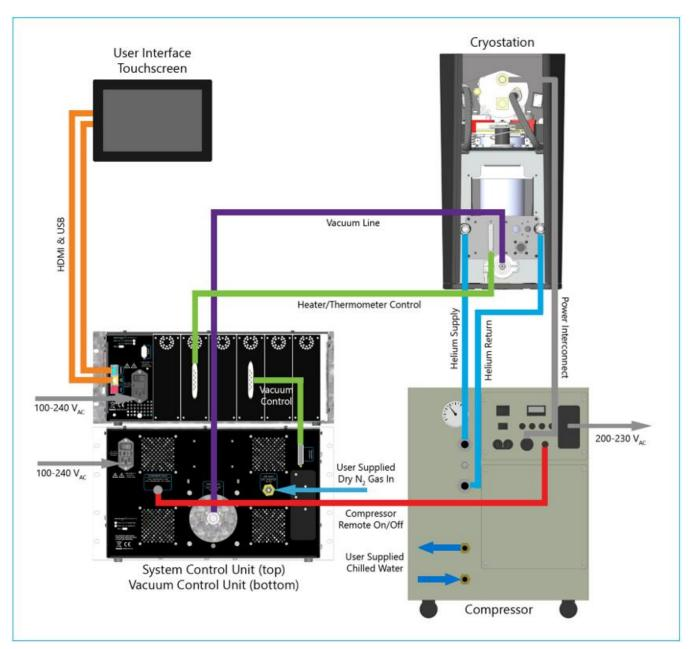
Figure 3: Cryostation interconnect diagram - F20-L compressor.
