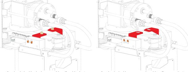
Bracket bolted in the lower position (for shipping)
