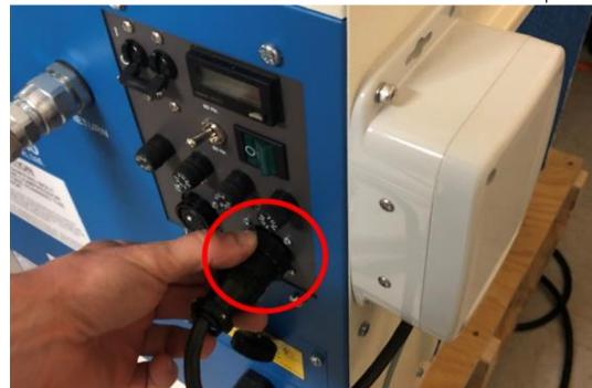
d. Connect the short cable to the ACCESSORY location on the front of the compressor
