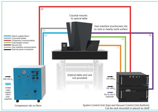
Figure 1: Component placement and layout.
