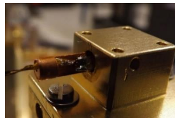
Step 3c: Thermometer installed in plug
