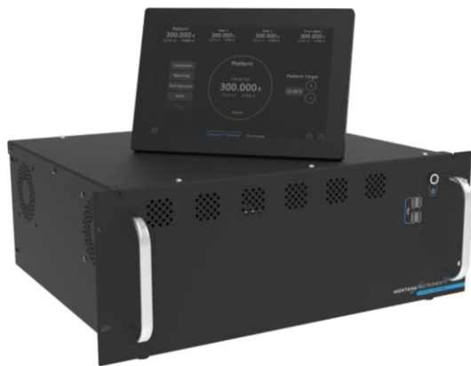
System Control Unit with User Interface Touchscreen
