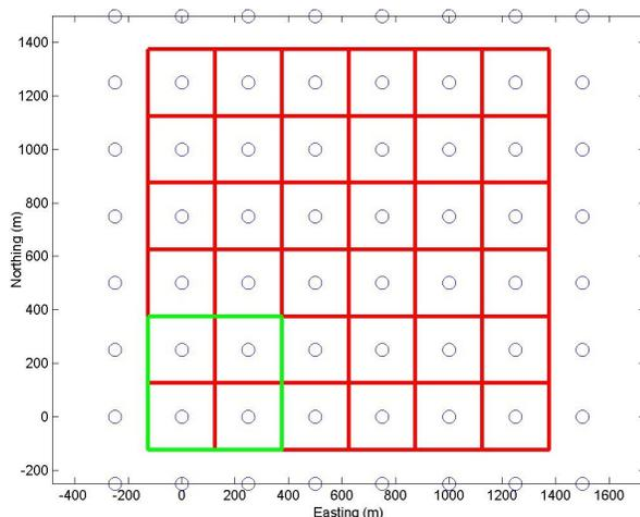
Figure 2: Survey geometry: 25 overlapping transmitter loops (red) on a  $5 \times 5$  grid. A single transmitter loop is highlighted in green, showing the 50% overlap of each transmitter loop. The 64 receivers (blue circles) are on a  $8 \times 8$  grid.
