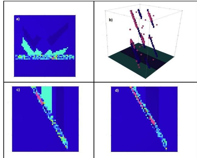
Figure 1: Synthetic conductivity model: pink is conductive, dark blue is resistive. a) Surface view. b) Showing only most conductive and resistive units. c) and d) Cross sections through the model.
