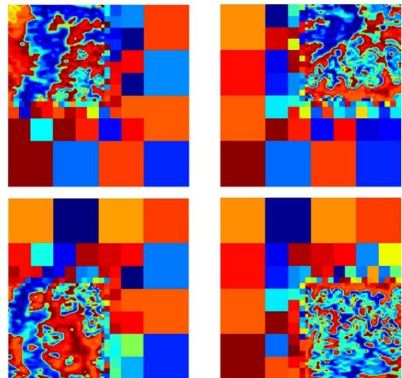
Figure 2: **Left:** Partitioning scheme used to invert the 350 x 450 km block of VTEM data collected by Geoscience BC as part of the QUEST project. **Right:** Resulting discretization of model in Figure 1 using four sub-domain OcTree meshes.
