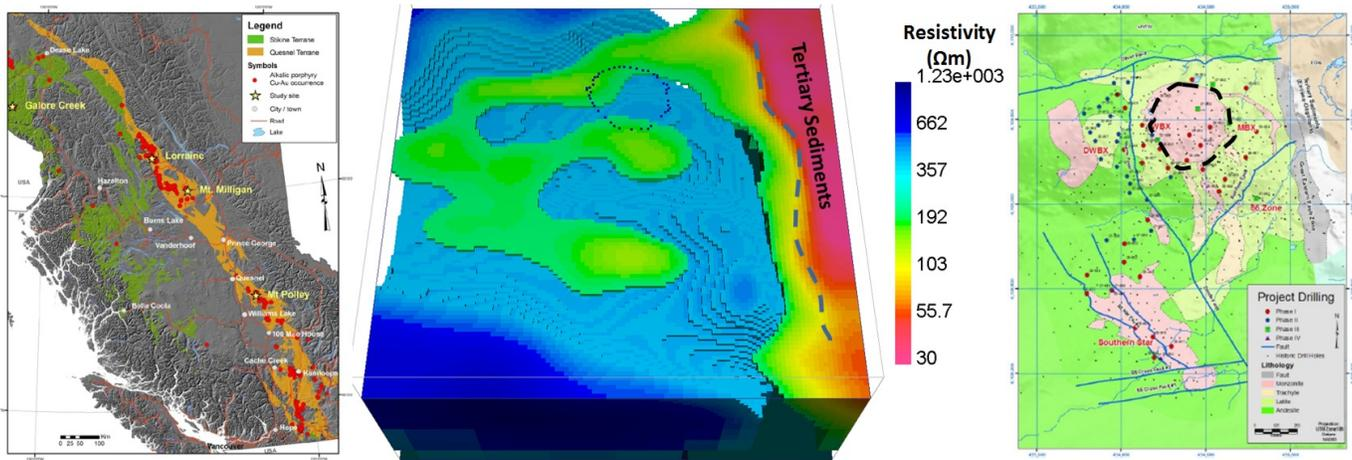
Figure 3: **Left:** Mt. Milligan location in British Columbia in the Quesnel Terrane (Devine, 2011). **Center:** Inverted VTEM conductivity model at an elevation of 965 m showing the more conductive and resistive units. **Right:** Mt. Milligan general geology taken from the 2009 Terrane Metals Corp. 43-101 report.
