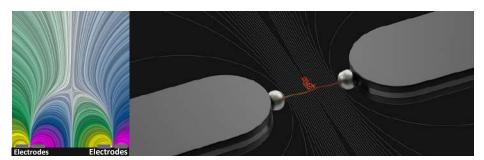
The electric field created by the sensor nano-electrodes (left) can be used to produce a general attractive force (dielectrophoresis) that pulls molecules to the vicinity of the electrode gap. This effect is currently used to rapidly assemble the sensor (right) and enables the ability to pull targets to the sensor, increasing the limits of sensitivity.
