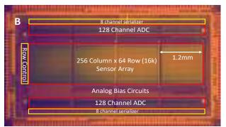
(Left) Annotated die image for the 16k CMOS sensor array chip. The 16k pixel array is organized as 4 banks of 4k pixels.
