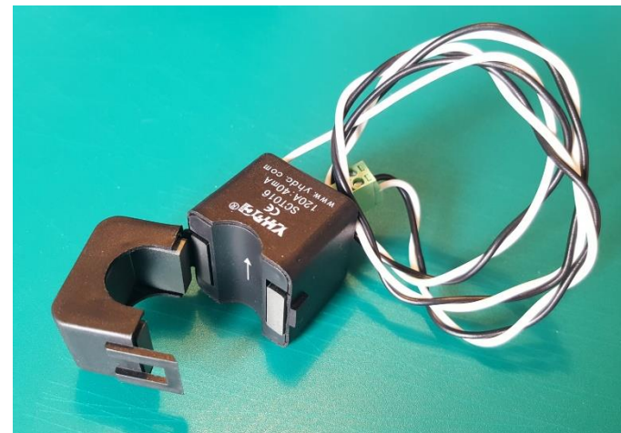
Picture 3 Current sensor. The arrow must indicate the direction of current (towards the house).
