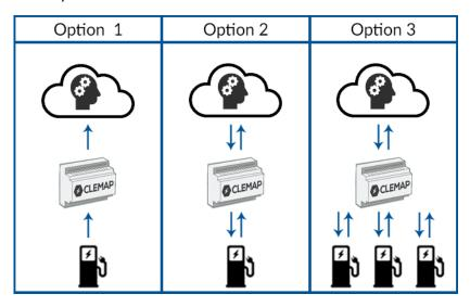
To send commands for dynamic load reduction to the charging stations, control signals via Modbus TCP were used. These were oriented to the maximum permissible amount of current and thus ensured uninterrupted charging.
