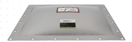
OsecoElfab's CRVC vent is a rectangular, domed explosion vent. The heavy-duty design incorporates much thicker materials than standard explosion vents. The CRVC can withstand higher positive or negative system operating pressures than flat vents. Positive system pressure should be limited to 70% of set pressure (Pstat).
