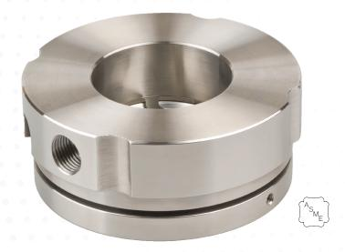
OsecoElfab's OPR/OPK Holder is designed for the OPR+/OPK+ rupture disc. It is available with taps for an excess flow valve or pressure gauge and for the non-invasive, re-usable Flo-Tel+ burst sensor.
