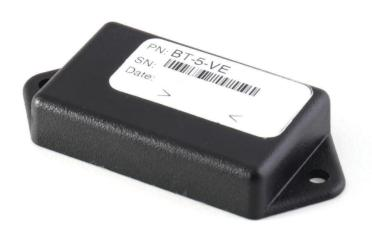
**SPECIFICATIONS Power Requirements** Internal Battery - Non-replaceable **Battery Extended Temperature Lithium Battery Life** Up to 2 years -40° to +70° C **Operating Temperature IP Rating** IP67 **Bluetooth Distance** Up to 100 yards - Line of Sight 2.45GHz, 802.15.4 Compliant **Bluetooth Frequency Dimensions** 2.08" x 1.28" x .45"
