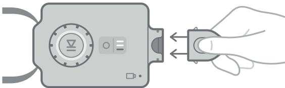
**Figure 4.** Connecting Garment to Controller.
