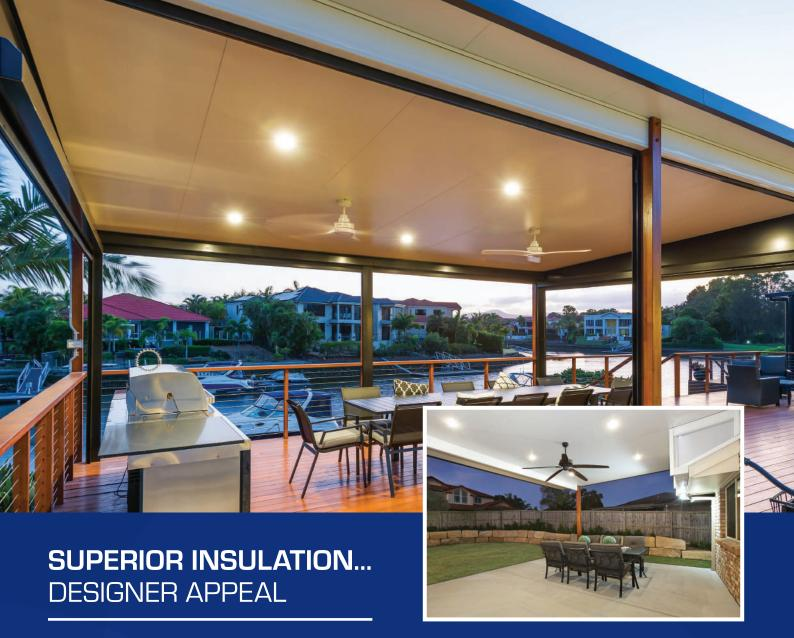
Your custom designed Ausdeck roofing comes with your choice of 50mm, 75mm, 100mm, 125mm or 150mm fire retardant insulated core: a roofing solution that reduces heat transmission and insulates against noise from rain and storms. This energy efficient insulation keeps your outdoor living area cool in summer and warmer in winter.
