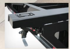
Container Locks on reinforced bolsters are positioned to handle two 8 ft, one 10 ft sand bin with ease.
