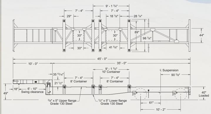
Estimated Weight: Base Models and standard specs from 8,700# to 8,950#
