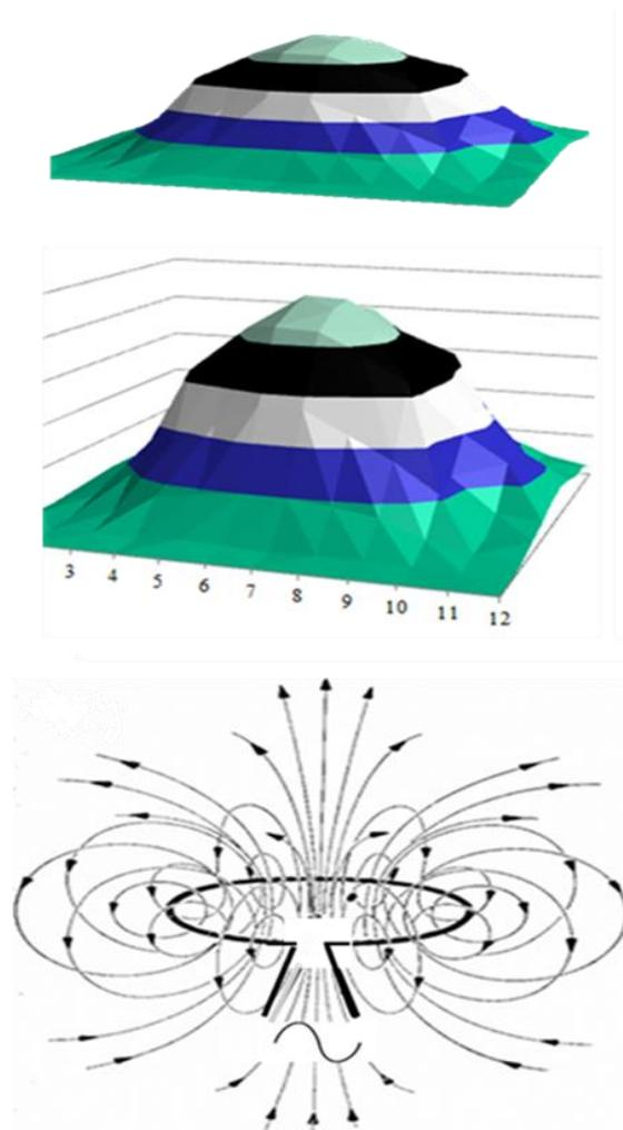
**Fig.3: 3-D field distribution (magnetic flux density) around a ring-shaped air-core coil.** The field intensity is strongly dependent on the distance to the coil surface. In the schematic example, each at a vertical distance of 0 and 15cm.
