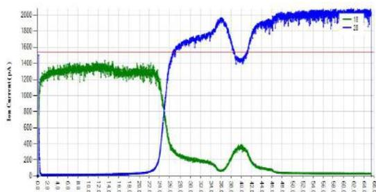
Figure 4 - Primary and secondary drying cycles as added N<sub>2</sub> replaces H<sub>2</sub>O to control the ambient pressure & hence the ice temperature.
