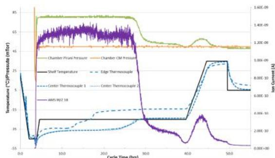
Figure 5 - Freeze drying of 5% w/v sucrose placebo.
