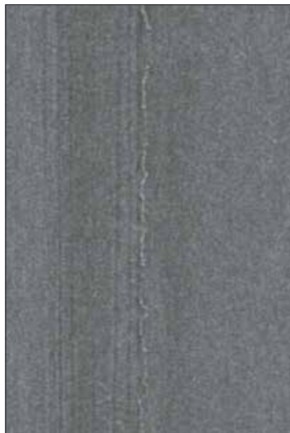
Fig 2: Sliver defect on galvanized strip
