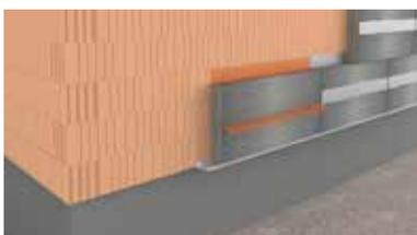
**1. A1 fire rated compartmentalisation** - The FSC has built-in A1 fire barriers that generate fire safe partitions within the insulation panel. These barriers prevent direct fire exposure inside the system and restrict the melted polystyrene foam from running down to the fire source and fuelling the fire.
