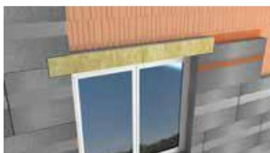
**2. Innovative window & door head fire barriers** - The FSC-EWI system requires that a specially modified mineral wool fire barrier is installed above all window and door heads. This pioneering fire barrier has been developed to prevent the absorption of melted polystyrene foam.
