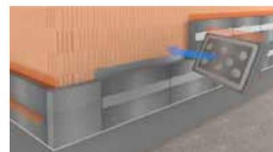
**3. Mechanically & wet fixed** - Composite panels are both mechanically and adhesively fixed. The insulation is glued to the substrate with A1 rated Soltherm adhesive. This adhesive prevents the movement of fire and toxic gasses behind the system.
