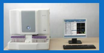
> Laser light multi-dimensional cell classification Resistant RBC mode WIC and WOC for WBC counting Up to 60 samples per hour throughput WBC 5 part diff with sheath reagent only Support both whole blood and capillary blood samples Four reagents for 25 parameters
