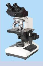
➤ Sliding binocular head, inclined at 45°
