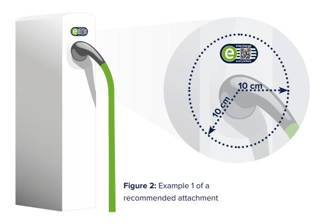
Basically we recommend two different ways of the placement: either in immediate proximity to the charging outlet or on the front or back of the charging station.
