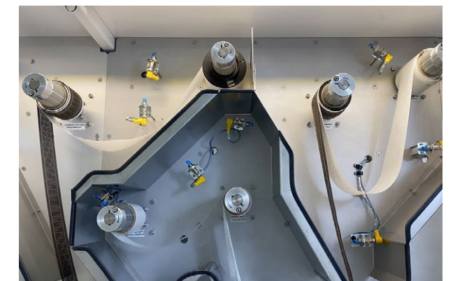
Photograph of electrode and separator rolls on proprietary roll-to-stack tool (source: Enovix Corporation)
