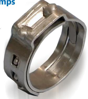
Many of our Pex (PEX) and Seamless (KVGT) clamps and Keystone (KSC) offer our patented crimp lobe technology. This feature ensures that the crimping tool is properly positioned to help eliminate miscrimps. Miscrimps often lead to leaks.
