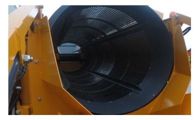
5'x16' Drum, Variable Screening Angle, Hopper Capacity: 3.8M³, Feeder Belt Width 950mm, Side Conveyor Belt Width 650mm, Transfer Conveyor Belt Width 1050mm, Oversize Conveyor Belt Width 950mm, Chevron Belt, Power Unit: CAT 4.4 74KW Engine, Tracks: 2.9M Tracks \* 300mm Shoes, Remote Control Movement
