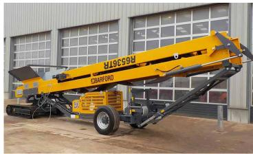
Radial Tracked Stockpile Conveyor 65ft x 36", Hydraulic Drive Slewing Wheels, Crawler Tracks at Feed Hopper, Rubber Lined Feed Hopper. Hydraulic Raise/Lower. Galvanized Inner Telescopic Legs. Galvanized Roller Guards. Cat 2.2 Engine
