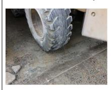
FEL parked with rear wheel in drain. This will assist to prevent a rollaway in the event of a brake failure.
