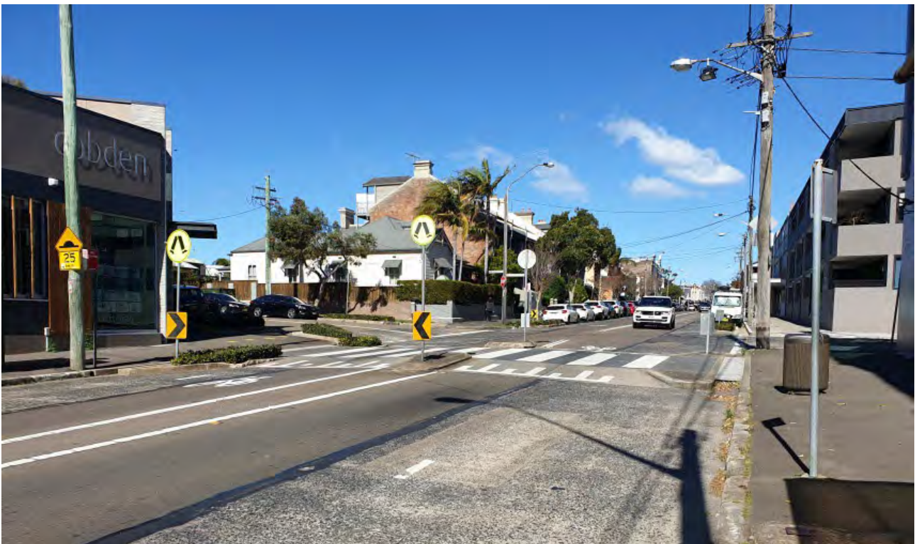
Figure B 21: Local Street wombat crossing, in combination with a pedestrian refuge and a kerb blister, set in a 40 km/h area-wide speed zone (Darling Street Rozelle, Sydney)
