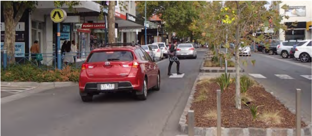
Figure B 37: Medians reduce the risk of pedestrian crashes (note scope for tree planting and public seating, subject to adequate median width)
