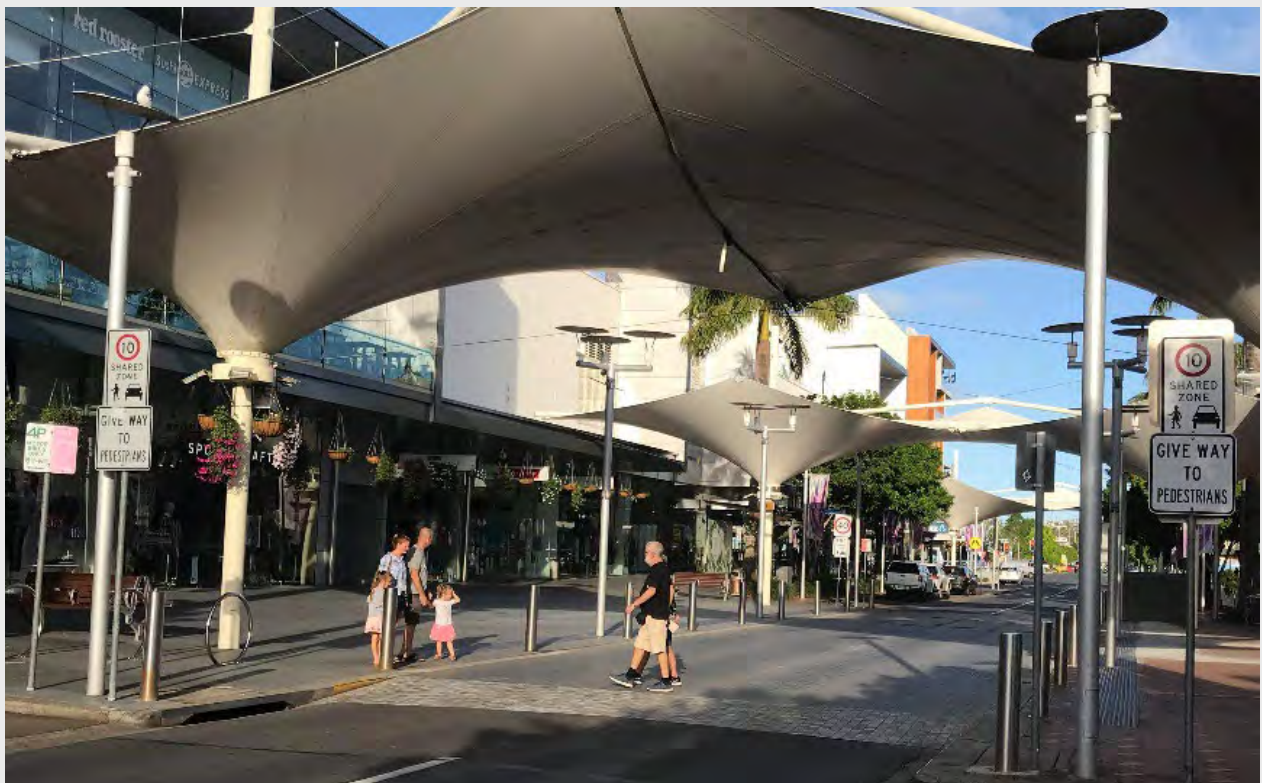
Figure 4.29: Shared space and shade sails combine to moderate speeds where pedestrian crossing activity is most concentrated (Coffs Harbour, New South Wales)
