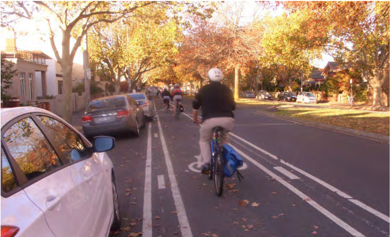
Figure B 33: Bicycle lane with adequate clearance to opened car doors – Melbourne suburb of Carlton
