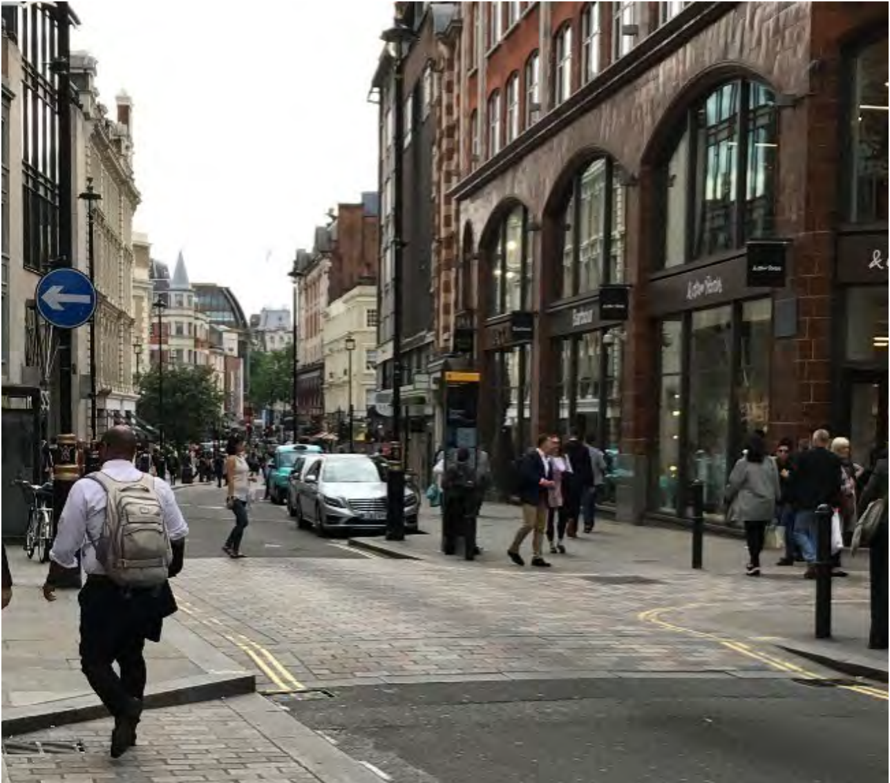
Figure B 23: Kerb blisters with safety platforms in a 20 mph city street in London
