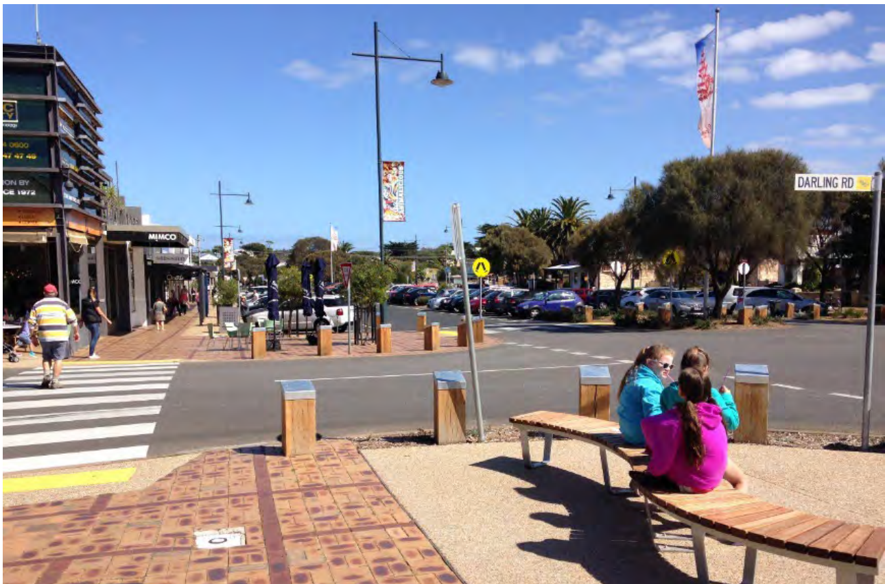
Figure B 22: Kerb blisters and zebra crossing (which can include provision for seating, cycle parking and street beautification)
