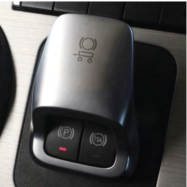
Parking brake, electronic. The electronic parking brake combines simple handling, driving comfort and safety.
