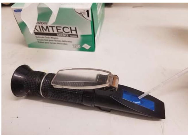
Example of applying a couple of drops of water to the reading window.
