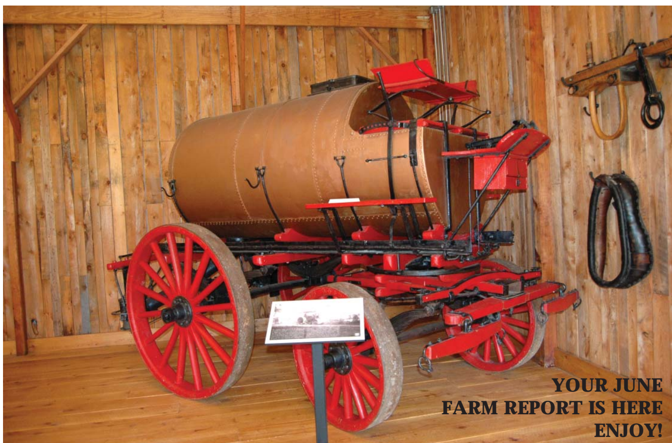
This vehicle is part of the antique vehicle exhibit in the Heart's Delight Farm Heritage Exhibit Coach House. It sprinkled water on the roads to keep the dust down at Heart's Delight Farm.
